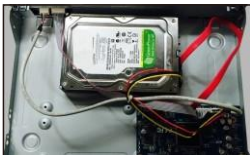
④ Connect the power and data cables.
