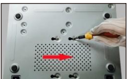
⑤ Turn over the machine and secure the HDD with the screws.
